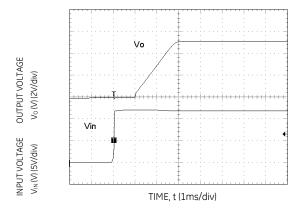
Figure 36. Typical Start-up Using Input Voltage ( $V_{IN} = 12V$ ,  $I_0 = I_{0,max}$ ).
