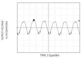
Figure 15. Typical output ripple and noise ( $V_{IN} = 12V$ ,  $I_0 = I_{O,mov}$ )
