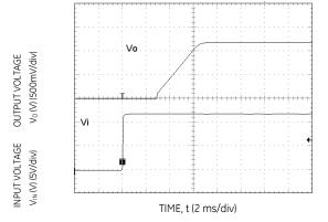
Figure 12. Typical Start-up Using Input Voltage ( $V_{IN} = 12V$ ,  $I_0 = I_{0,max}$ ).
