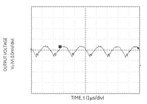
Figure 3. Typical output ripple and noise ( $V_{IN} = 12V$ ,  $I_0 = I_{0,max}$ ).
