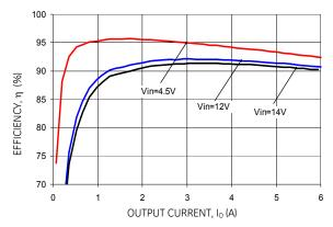
Figure 25. Converter Efficiency versus Output Current.
