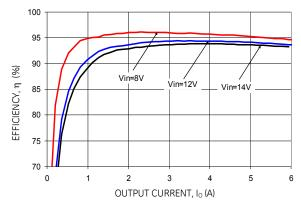
Figure 31. Converter Efficiency versus Output Current.
