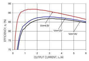
Figure 13. Converter Efficiency versus Output Current.
