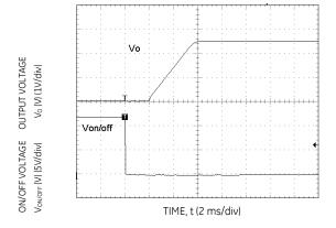
Figure 23. Typical Start-up Using On/Off Voltage ( $I_0 = I_{o,max}$ ).
