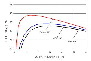
Figure 7. Converter Efficiency versus Output Current.
