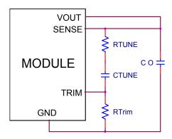
Figure. 48. Circuit diagram showing connection of  $R_{\text{TUME}}$  and  $C_{\text{TUNE}}$  to tune the control loop of the module.
