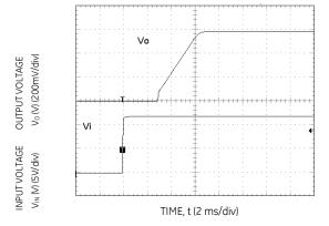
Figure 6. Typical Start-up Using Input Voltage ( $V_{IN} = 12V$ ,  $I_0 = 1...$
