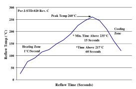
Figure 51. Recommended linear reflow profile using Sn/Ag/Cu solder.
