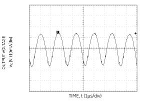
Figure 21. Typical output ripple and noise ( $V_{IN} = 12V$ ,  $I_0 = I_{0,max}$ ).
