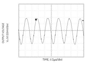
Figure 27. Typical output ripple and noise ( $V_{IN} = 12V$ ,  $I_0 = I_{0,max}$ ).
