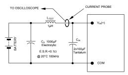
NOTE: Measure input reflected ripple current with a simulated source inductance ( $L_{\text{TEST}}$ ) of 1 $\mu$ H. Capacitor  $C_{\text{S}}$  offsets possible battery impedance. Measure current as shown above.
