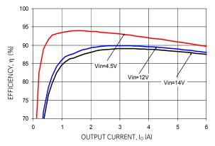
Figure 19. Converter Efficiency versus Output Current.
