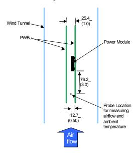
Figure 49. Thermal Test Setup.
