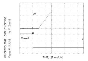
Figure 33. Typical Start-up Using On/Off Voltage ( $I_0 = I_{o,max}$ ).
