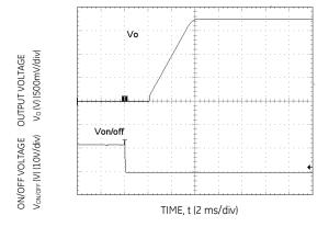
Figure 17. Typical Start-up Using On/Off Voltage ( $I_0 = I_{o,max}$ ).
