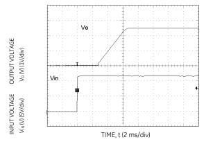
Figure 24. Typical Start-up Using Input Voltage ( $V_{IN} = 12V$ ,  $I_0 = I_{o,max}$ ).
