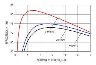
Figure 1. Converter Efficiency versus Output Current.
