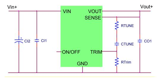
CI1  $22\mu\text{F}/16\text{V}$  ceramic capacitor (e.g. Murata GRM32ER61C226KE20)
