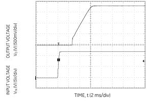
Figure 18. Typical Start-up Using Input Voltage ( $V_{IN} = 12V$ ,  $I_0 = I_{0,max}$ ).
