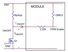
Figure 42. Circuit configuration for using positive On/Off logic.
