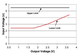
Figure 39. Output Voltage vs. Input Voltage Set Point Area plot showing limits where the output voltage can be set for different input voltages.
