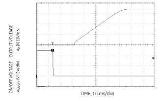
Figure 29. Typical Start-up Using On/Off Voltage ( $I_0 = I_{0,max}$ ).
