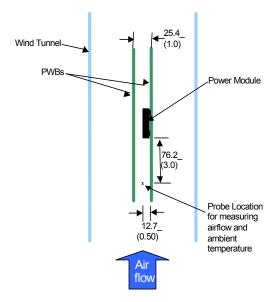
Figure 44. Thermal Test Setup.
