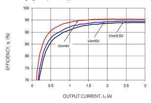
Figure 25. Converter Efficiency versus Output Current.
