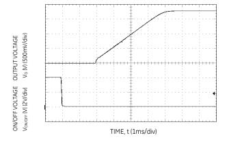
Figure 17. Typical Start-up Using On/Off Voltage ( $I_0 = I_{0,max}$ ).
