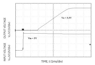
Figure 30. Typical Start-up Using Input Voltage ( $V_{IN} = 5V$ ,  $I_0 = I_{0,max}$ ).
