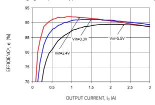
Figure 7. Converter Efficiency versus Output Current.
