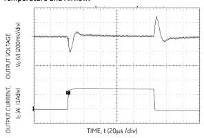
Figure 28. Transient Response to Dynamic Load Change from 0% 50% to 0% with  $V_{\text{IN}}$ =5V.
