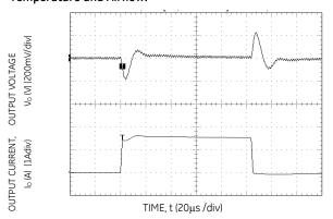
Figure 16. Transient Response to Dynamic Load Change from 0% to 50% to 0% with  $V_{\text{IN}}$ =5V.
