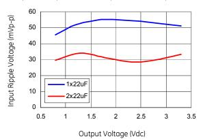
Figure 34. Input ripple voltage for various output voltages with 1x22  $\mu F$  or 2x22  $\mu F$  ceramic capacitors at the input (3A load). Input voltage is 5V.
