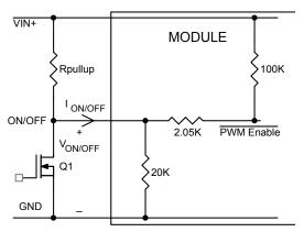
Figure 38. Circuit configuration for using negative On/Off logic.
