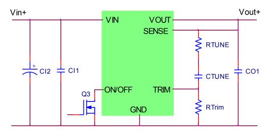
CI1  $22\mu\text{F/6.3V}$  ceramic capacitor CI2  $47\mu\text{F/6.3V}$  bulk electrolytic
