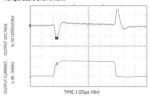
Figure 4. Transient Response to Dynamic Load Change from 0% to 50% to 0% with  $V_{\rm IN}{=}5V$ .
