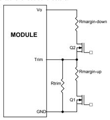
Figure 41. Circuit Configuration for margining Output voltage
