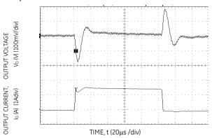
Figure 10. Transient Response to Dynamic Load Change from 0% to 50% to 0% with  $V_{\rm IN}$ =5V.
