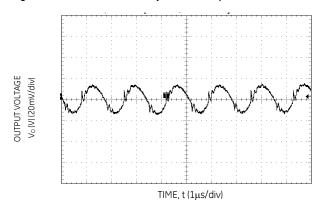
Figure 15. Typical output ripple and noise ( $V_{IN} = 5V$ ,  $I_0 = I_{0,max}$ ).
