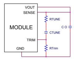
Figure. 43. Circuit diagram showing connection of  $R_{\text{TUME}}$  and  $C_{\text{TUNE}}$  to tune the control loop of the module.
