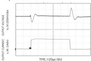
Figure 22. Transient Response to Dynamic Load Change from 0% to 50% to 0% with  $V_{\text{IN}}$ =5V.
