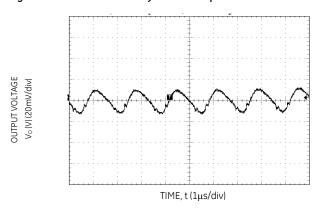
Figure 9. Typical output ripple and noise ( $V_{IN} = 5V$ ,  $I_0 = I_{o,max}$ ).
