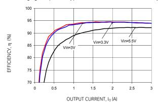
Figure 19. Converter Efficiency versus Output Current.
