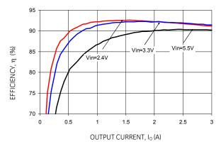
Figure 13. Converter Efficiency versus Output Current.
