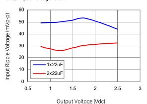
Figure 35. Input ripple voltage in mV, p-p for various output voltages with 1x22  $\mu$ F or 2x22  $\mu$ F ceramic capacitors at the input (3A load). Input voltage is 3.3V.
