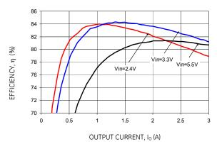
Figure 1. Converter Efficiency versus Output Current.
