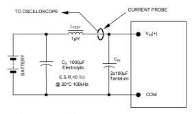
NOTE: Measure input reflected ripple current with a simulated source inductance ( $L_{\text{TEST}}$ ) of 1µH. Capacitor  $C_{\text{S}}$  offsets possible battery impedance. Measure current as shown above.
