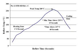
Figure 46. Recommended linear reflow profile using Sn/Ag/Cu solder.
