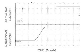
Figure 36. Typical Start-up Using Input Voltage ( $V_{IN}=12V,\ I_0=I_{0,max},\ Cext=22uF$ ).
