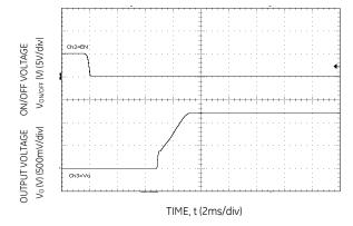
Figure 11. Typical Start-up Using On/Off Voltage ( $I_0 = I_{0,max}$ ,  $V_{in=12V,Cext=22uF$ ).
