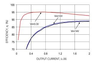
Figure 19. Converter Efficiency versus Output Current.
