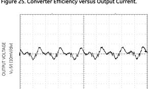
Figure 27. Typical output ripple and noise ( $V_{IN} = 12V$ ,  $I_0 =$ lo,max).
