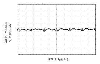
Figure 3. Typical output ripple and noise ( $V_{IN} = 12V$ ,  $I_0 = I_{O,max}$ ).
