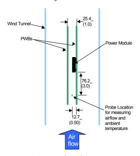
Figure 48. Thermal Test Setup.
