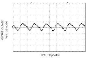
Figure 33. Typical output ripple and noise ( $V_{IN} = 12V$ ,  $I_0 = I_{0,max}$ ).
