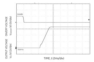
Figure 29. Typical Start-up Using On/Off Voltage (Io = Io,max, Vin=12V,Cext= 22uF)
