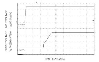
Figure 12. Typical Start-up Using Input Voltage ( $V_{IN} = 12V$ , Cext = 22uF,  $I_0 = I_{0,max}$ ).
