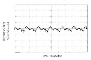
Figure 15. Typical output ripple and noise ( $V_{IN} = 12V$ ,  $I_0 = I_{0,max}$ ).
