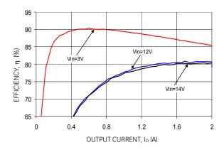
Figure 7. Converter Efficiency versus Output Current.
