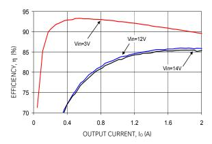
Figure 13. Converter Efficiency versus Output Current.
