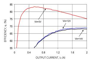
Figure 1. Converter Efficiency versus Output Current.
