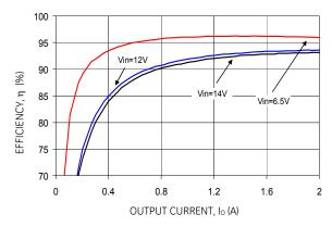
Figure 31. Converter Efficiency versus Output Current.
