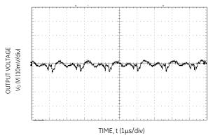
Figure 9. Typical output ripple and noise ( $V_{IN}=12V$ ,  $I_0=I_{0,max}$ ).
