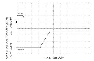
Figure 23. Typical Start-up Using On/Off Voltage ( $I_0 = I_{0,max}$ ,  $V_{in=12V,Cext=22uF}$ ).
