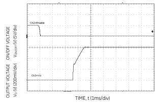
Figure 5. Typical Start-up Using On/Off Voltage ( $I_0 = I_{o,max}$ ,  $V_{in=12V,Cext=22uF}$ ).
