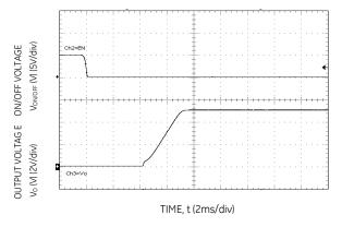
Figure 35. Typical Start-up Using On/Off Voltage ( $I_0 = I_{0,max}$ ,  $V_{in=12V,Cext=22uF$ ).
