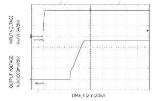
Figure 18. Typical Start-up Using Input Voltage ( $V_{IN} = 12V$ , Cext = 22uF,  $I_0 = I_{0,max}$ ).
