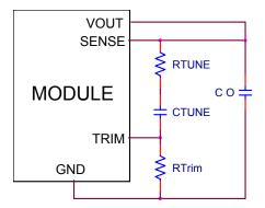
Figure. 47. Circuit diagram showing connection of  $R_{\text{TUME}}$  and  $C_{\text{TUNE}}$  to tune the control loop of the module.
