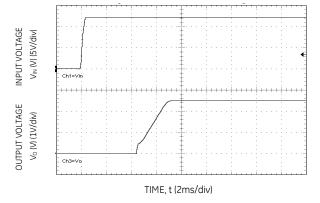
Figure 24. Typical Start-up Using Input Voltage ( $V_{IN} = 12V$ , Cext= 22 uF,  $I_0 = I_{0,max}$ ).
