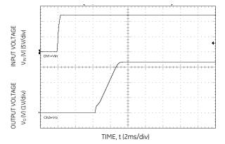
Figure 30. Typical Start-up Using Input Voltage (VIN = 12V, Cext= 22 uF,  $I_0 = I_{0,max}$ ).
