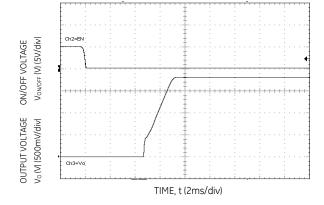
Figure 17. Typical Start-up Using On/Off Voltage ( $I_0 = I_{0,max}$ ,  $V_{in=12V,Cext=22uF,J}$ .
