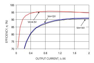
Figure 25. Converter Efficiency versus Output Current.
