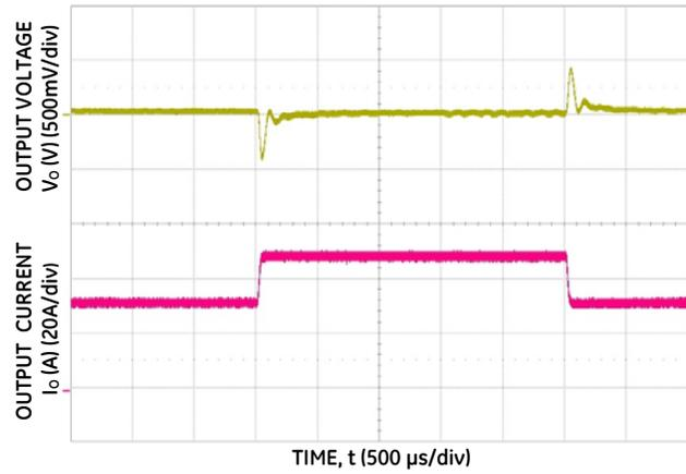
Figure 4. Typical Transient Response to 1.0A/µs Step Change in Load from 60% to 90% to 60% of Full Load,  $C_o=470\mu F$  and 50 V<sub>dc</sub> Input.
