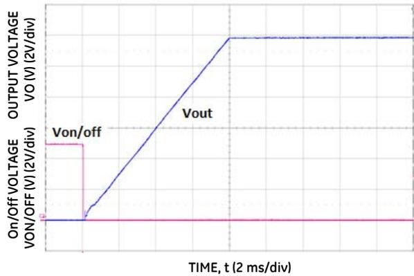
Figure 8. Typical Start-Up Using Remote On/Off with Vin applied, negative logic version, with the -P option shown,  $I_o = 33.5A$ .
