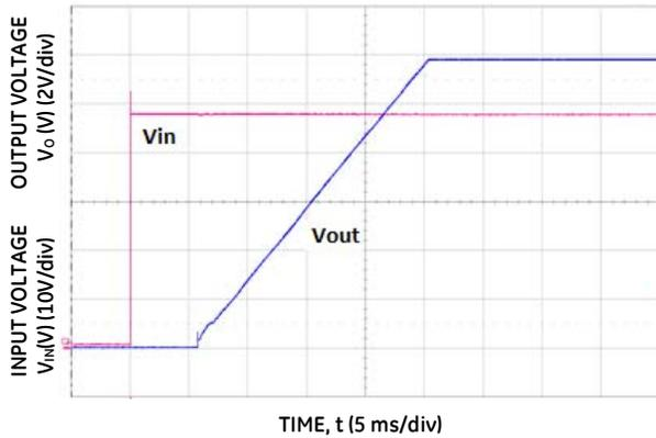
Figure 7. Typical Start-Up Using Vin with Remote On/Off enabled, negative logic version, with the -P option shown,  $I_o = 33.5A$ .
