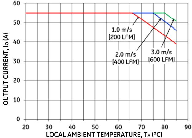
Figure 23. Output Current Derating for the Base Plate QBDE055A0Bxx-H+1.0" Heat Sink in the Transverse Orientation; Airflow Direction from Vin(-) to Vin(+); Vin = 50V.
