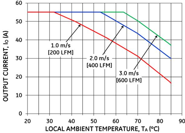
Figure 19. Output Current Derating for the Base Plate QBDE055A0Bxx-H in the Transverse Orientation; Airflow Direction from Vin(-) to Vin(+); Vin = 50V.
