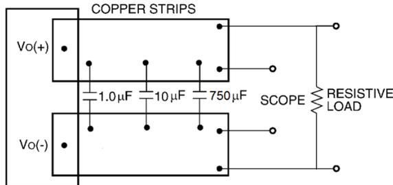
Note: Use a 1.0 µF ceramic capacitor, a 10 µF aluminum or tantalum capacitor and a 750 polymer capacitor. Scope measurement should be made using a BNC socket. Position the load between 51 mm and 76 mm (2 in. and 3 in.) from the module.
