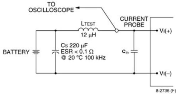
Note: Measure input reflected-ripple current with a simulated source inductance (LTEST) of 12 µH. Capacitor Cs offsets possible battery impedance. Measure current as shown above.
