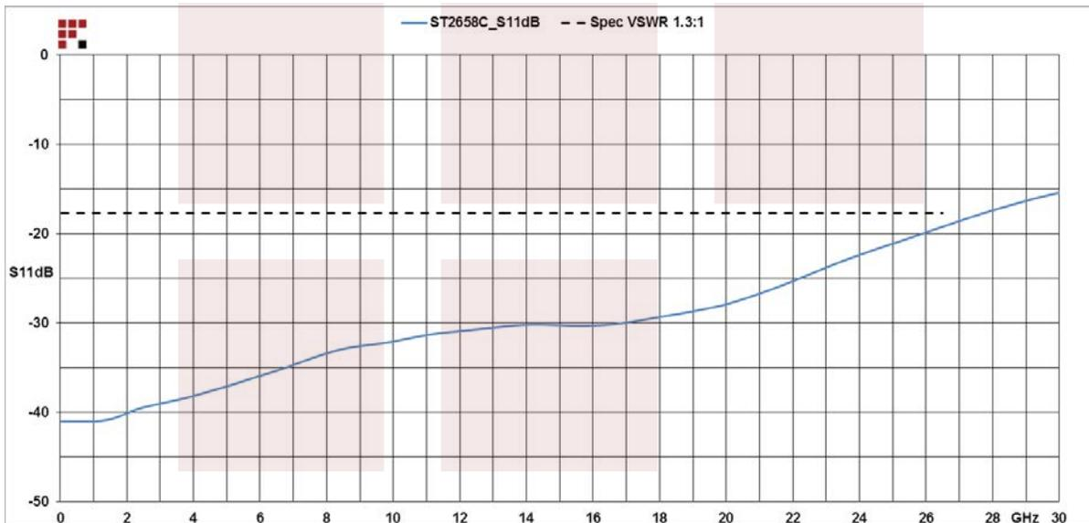
RF Load 1 Watts To 26.5 GHz With Chain Passivated Stainless Steel SMA Male from Fairview Microwave is in-stock and available to ship same-day. All of our RF/microwave products are available off-the-shelf from our ISO 9001:2008 certified facilities in Allen, Texas. Fairview Microwave is RF on-demand.
