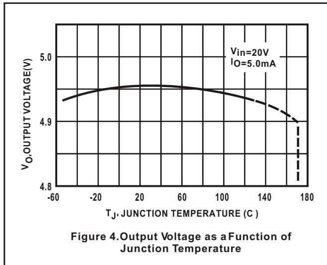
Figure 4. Output Voltage as a Function of Junction Temperature
