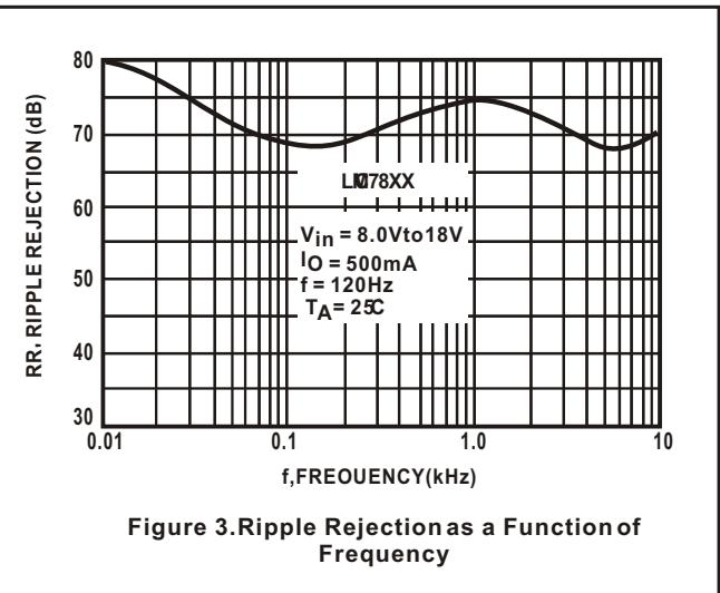
Figure 3. Ripple Rejection as a Function of Frequency
