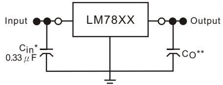
A common ground is required between the input and the output voltages. The input voltage must remain typically 2.0V above the output voltage even during the low point on the input ripple voltage.
