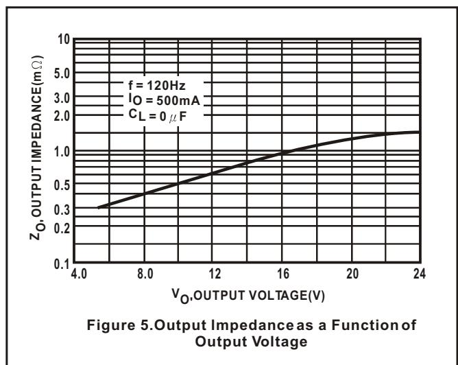
Figure 5. Output Impedance as a Function of Output Voltage
