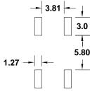
**Pin Connections** #1 E/D #3 Output #2 GND #4 V<sub>DD</sub>
