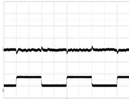
Output voltage response to load current step-change (3.5-10.5-3.5 A) at:
