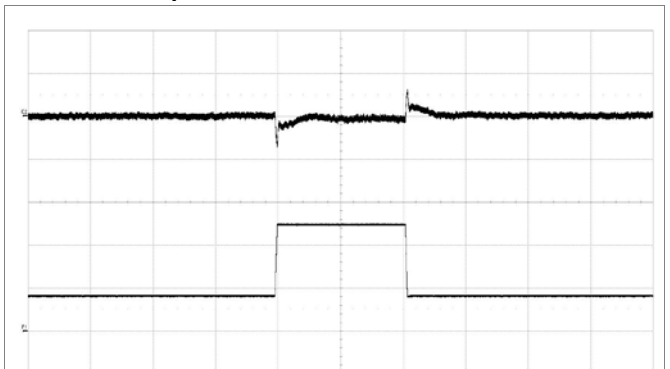
Output voltage response to load current step change (25%–75%–25%) at V_I = 12\text{ V} , C_{OUT} = 8 \times 330\text{ }\mu\text{F}/10\text{ m}\Omega + 20 \times 100\text{ }\mu\text{F} , di/dt = 2\text{ A}/\mu\text{s} , ACSR Gian=219 and ASCR Residual=82. Scale from top: 50 mV/div, 20 A/div, 500 \mu\text{s} /div. Note: Sense pins are connected to load.
