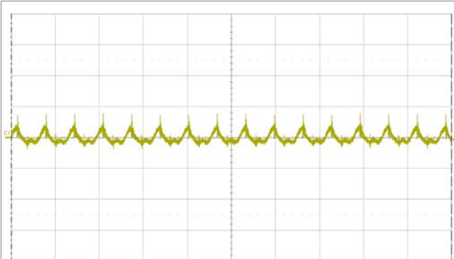
Output voltage ripple at: T_{P1} = +25^{\circ}\text{C} , V_I = 110\text{ V} , I_O = 8.4\text{ A} resistive load. Trace: output voltage (50 mV/div.). Time scale: (5 \mu\text{s} /div.). 20 MHz bandwidth.
