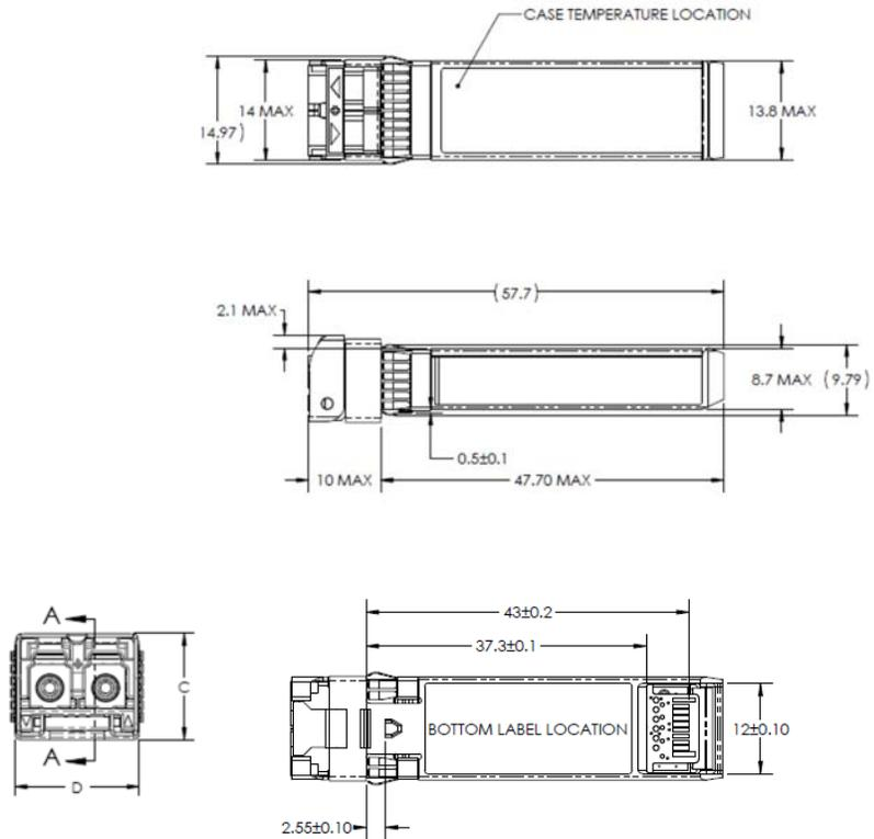
Figure 2. Mechanical Dimensions
