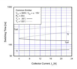
Fig 12. Turn-Off Characteristics vs. Collector Current
