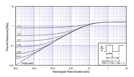
Fig 17. Transient Thermal Impedance of IGBT
