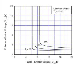
Fig 6. Saturation Voltage vs. V<sub>GE</sub>
