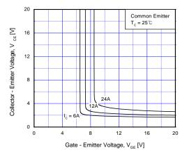
Fig 5. Saturation Voltage vs. V<sub>GE</sub>
