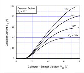
Fig 1. Typical Output Characteristics
