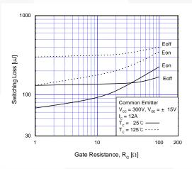
Fig 10. Switching Loss vs. Gate Resistance
