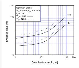
Fig 8. Turn-On Characteristics vs.
