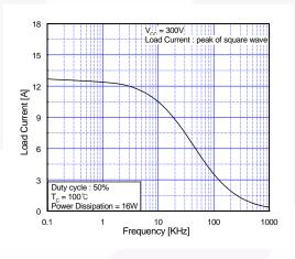
Fig 4. Load Current vs. Frequency
