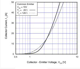
Fig 2. Typical Saturation Voltage Characteristics
