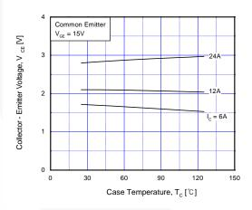
Fig 3. Saturation Voltage vs. Case
