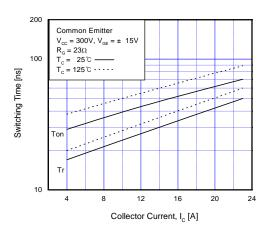
Fig 11. Turn-On Characteristics vs. Collector Current
