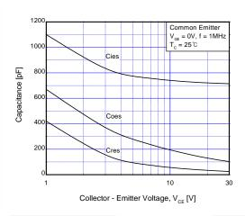
Fig 7. Capacitance Characteristics
