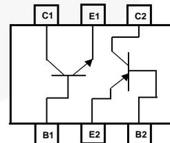
Figure 1. Block Diagram
