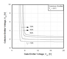
Figure 6. Saturation Voltage vs.  $V_{GE}$
