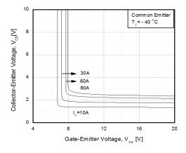
Figure 5. Saturation Voltage vs. V<sub>GE</sub>
