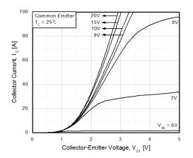
Figure 2. Typical Saturation Voltage Characteristics
