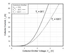
Figure 3. Saturation Voltage vs. Case
