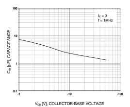
Figure 3. Output Capacitance
