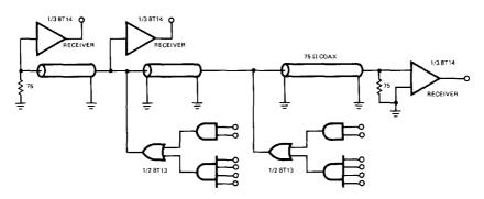
Note: For party line operation, termination of each physical end of the line is recommended.
