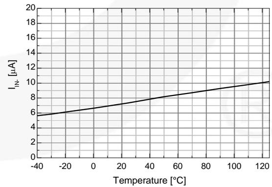
Figure 27. Logic Input LOW Bias Current vs. Temperature
