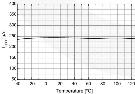
**Figure 14. Quiescent  $V_{DD}$  Supply Current vs. Temperature**
