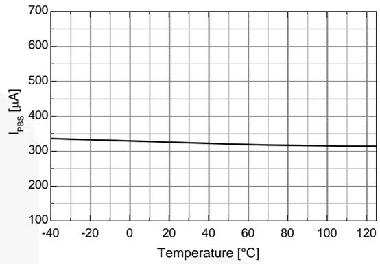
**Figure 17. Operating  $V_{BS}$  Supply Current vs. Temperature**
