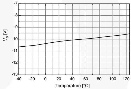
**Figure 13. Allowable Negative  $V_S$  Voltage vs. Temperature**
