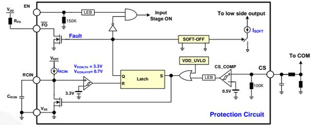
Figure 42. Over-Current Protection
