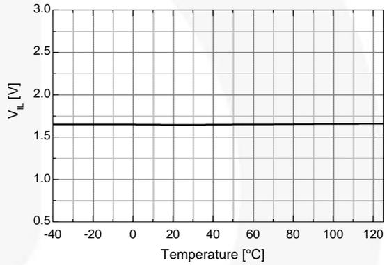
Figure 25. Logic LOW Input Voltage vs. Temperature
