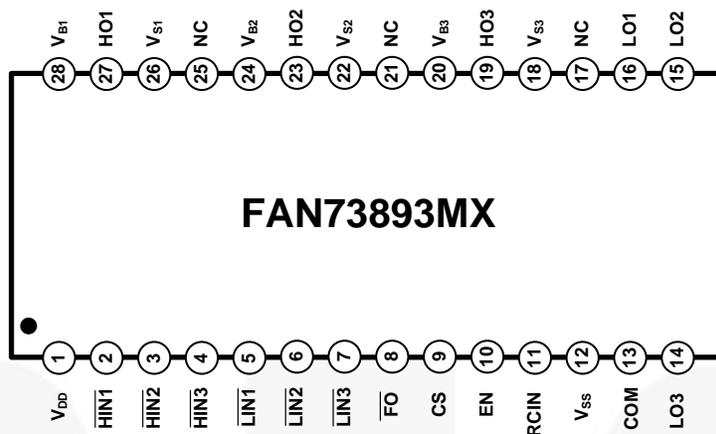
Figure 3. Pin Assignments
