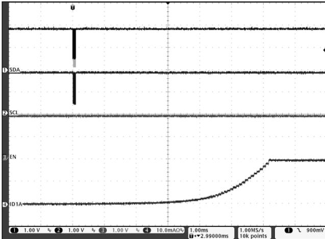
Figure 15. Linear Dimming via I<sup>2</sup>C Interface,  $V_{IN}=3.6\text{ V}$ ,  $I_{LEDx}=20\text{ mA}$ , and  $t_{RAMP}=6.4\text{ ms}$
