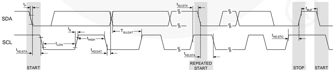
Figure 18. I<sup>2</sup>C Interface Timing for Fast and Slow Modes
