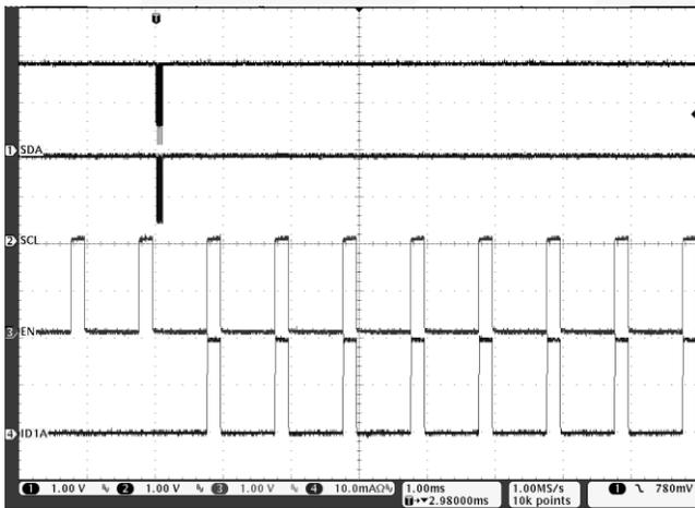
Figure 17. PWM and Linear (via I<sup>2</sup>C) Dimming,  $V_{IN}=3.6\text{ V}$ ,  $I_{LEDx}=20\text{ mA}$ , and  $EN=1\text{ kHz}$  with 20% Duty Cycle
