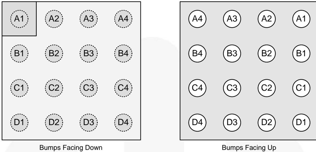
Figure 2. WLCSP-16, 0.4 mm Pitch, 1.61 x 1.61 mm
