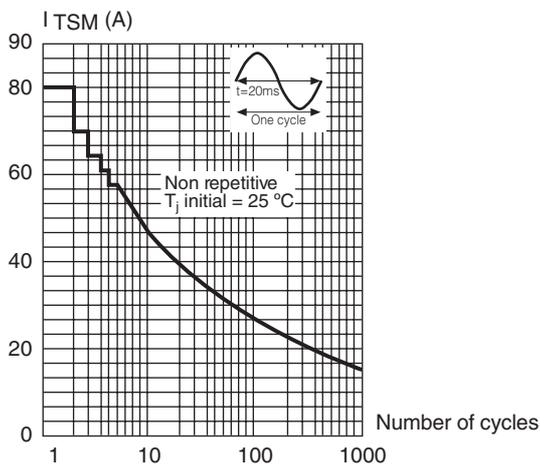
Fig. 6: Non repetitive surge peak on-state current for a sinusoidal pulse with width: tp < 10 ms, and corresponding value of I²t.
