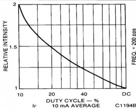
Fig. 3. Luminous Intensity vs. Duty Cycle
