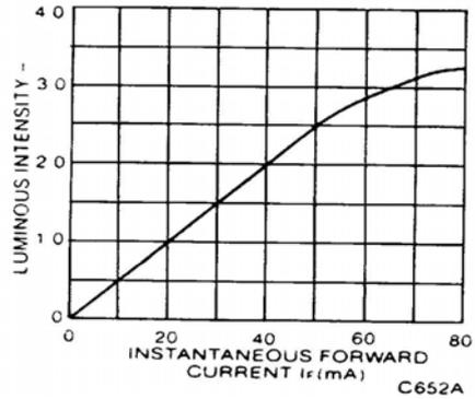
Fig. 2. Luminous Intensity vs. Forward Current
