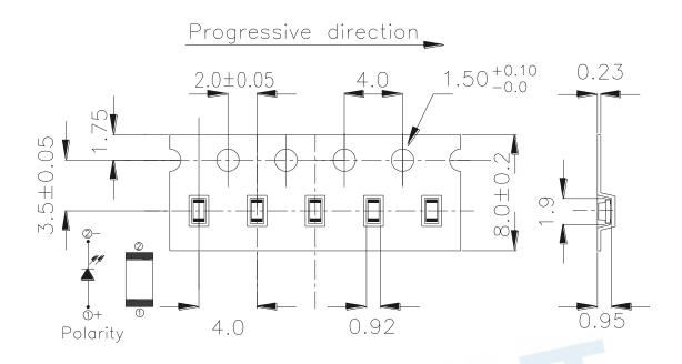
Note: The tolerances unless mentioned is  $\pm 0.1$ mm ,Unit = mm
