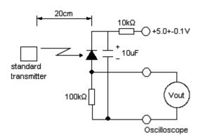
Fig.-3 Measuring System
