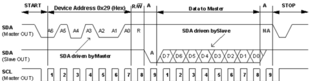
Figure 15. I<sup>2</sup>C Timing Diagram for Receive Byte Format
