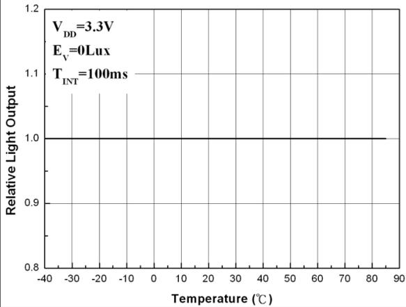
**Fig 10. Light Counts vs. Temperature**
