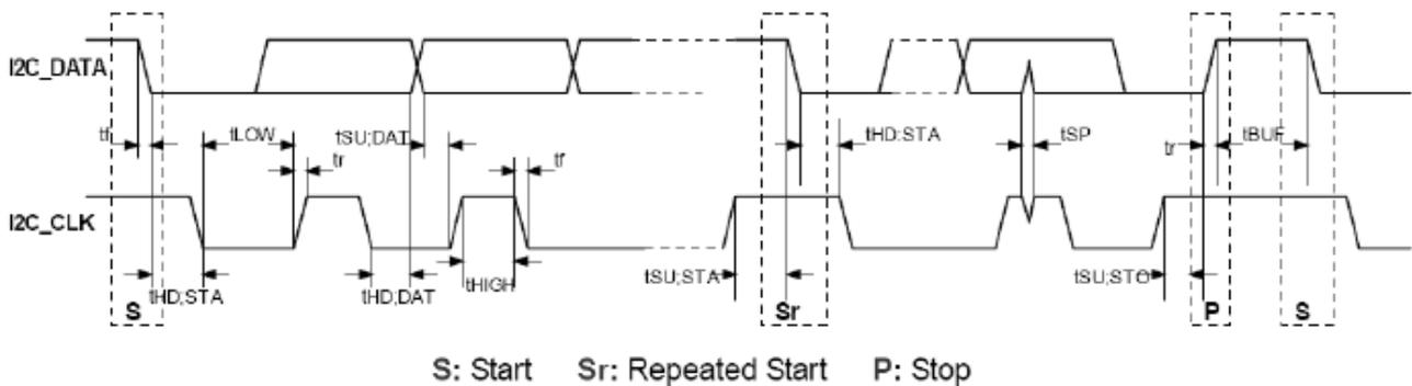
Figure 2. I<sup>2</sup>C Timing Diagram
