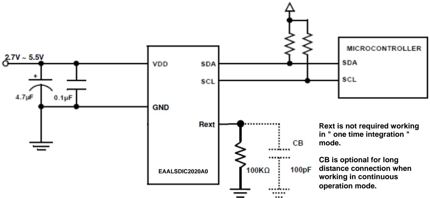
Figure 17. Application Circuit
