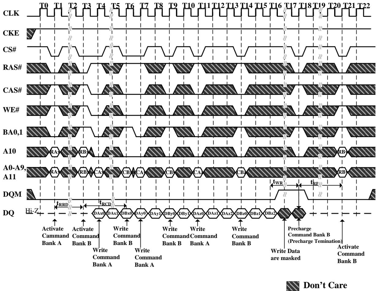
**Figure 42. Precharge Termination of a Burst**
