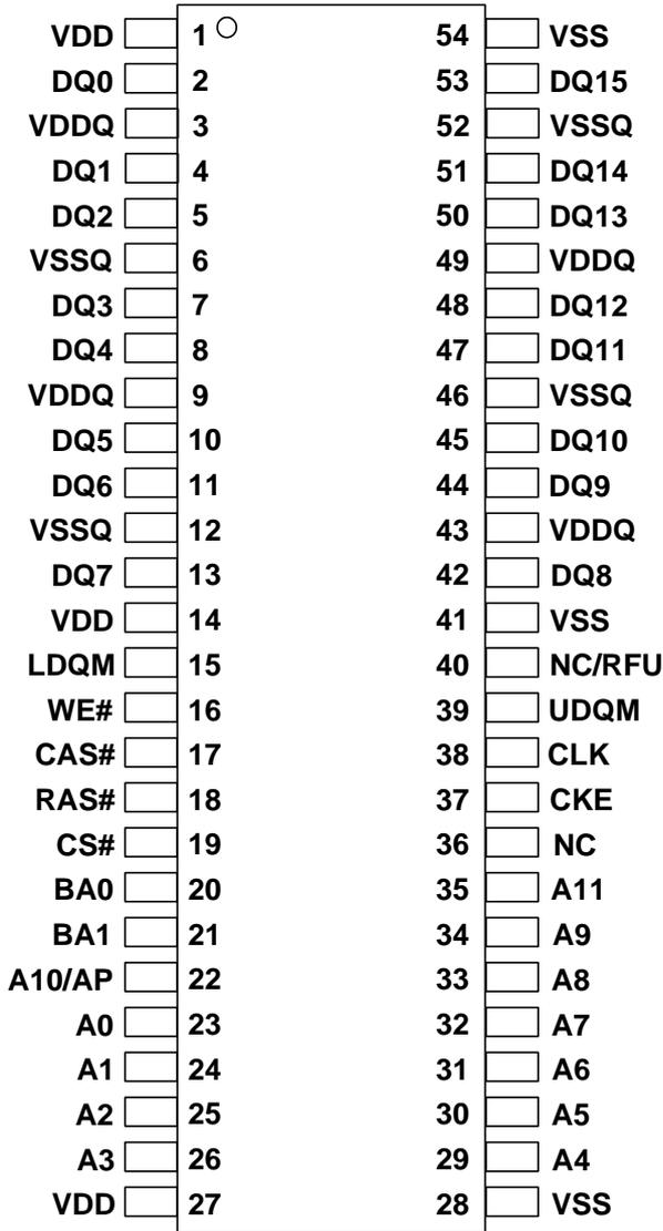
Figure 1.2 Ball Assignment (Top View)
