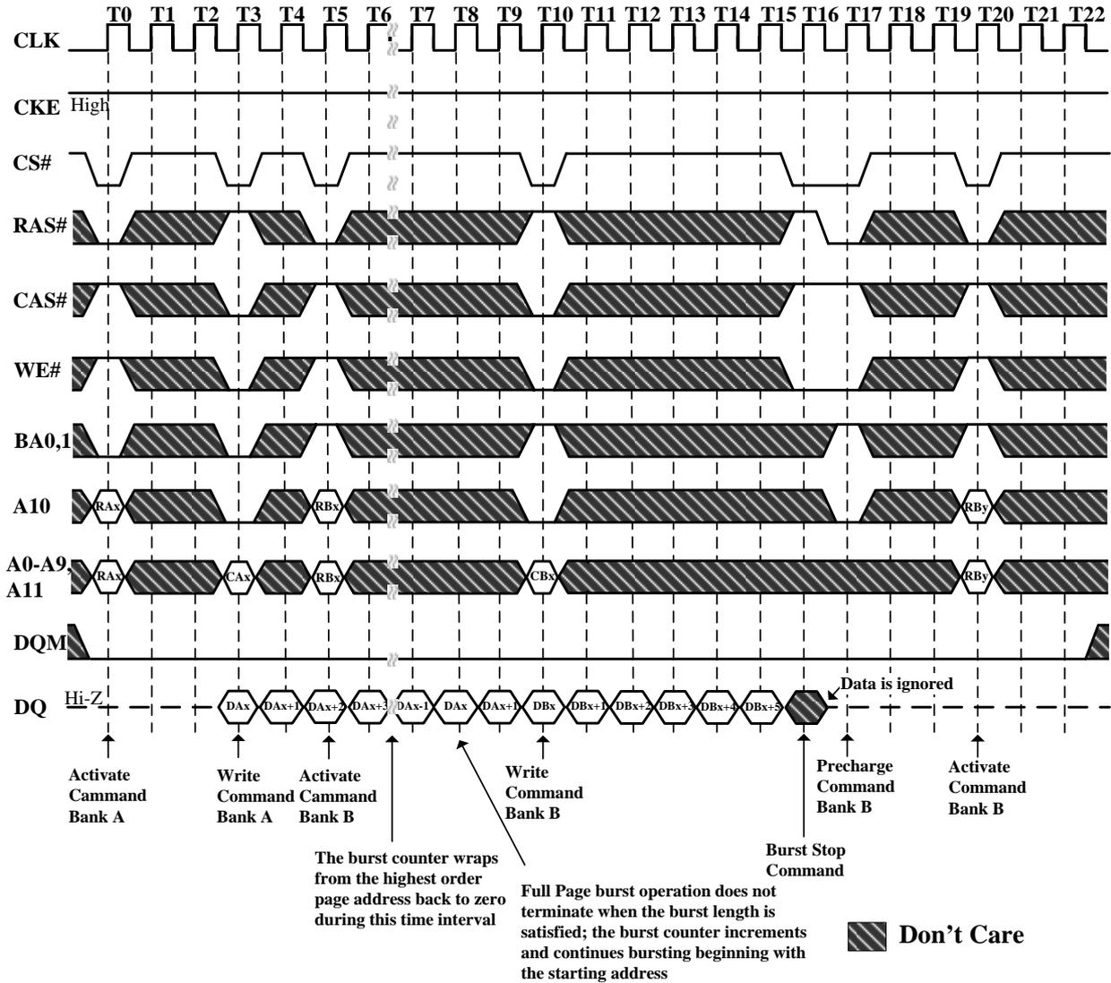
Figure 38. Byte Write Operation (Burst Length=4, CAS# Latency=2)
