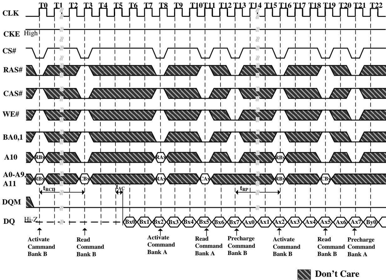
**Figure 30. Random Row Write (Interleaving Banks)**
