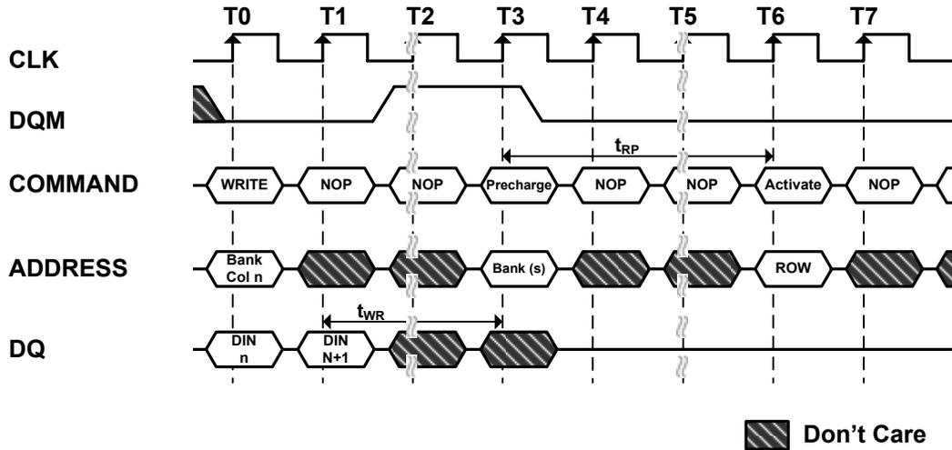
**Note:** The LDQM/UDQM can remain low in this example if the length of the write burst is 1 or 2.
