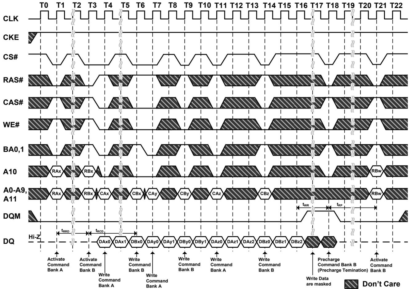
**Figure 42. Precharge Termination of a Burst**
