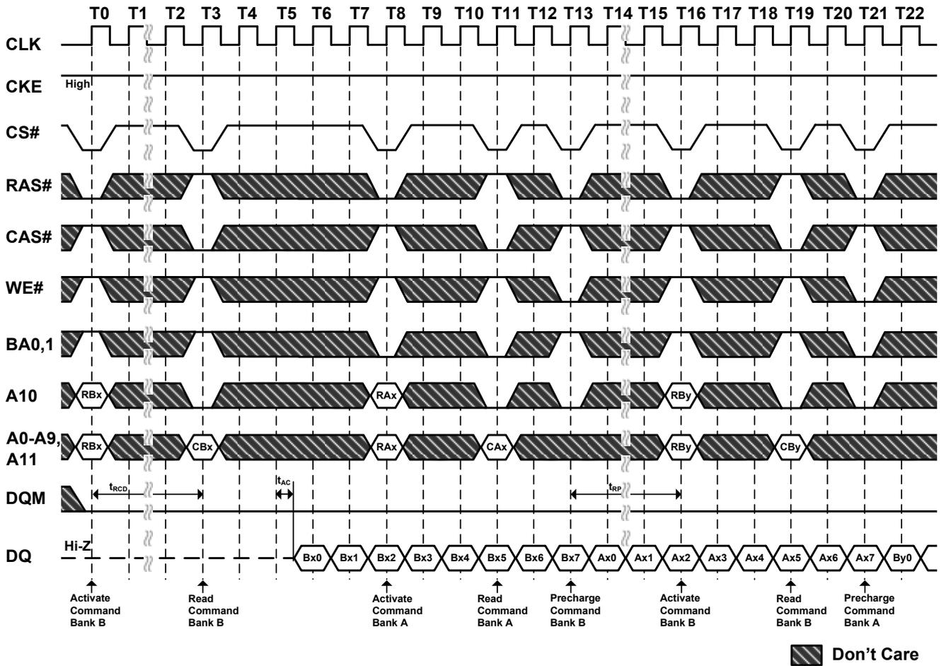
**Figure 30. Random Row Write (Interleaving Banks)**
