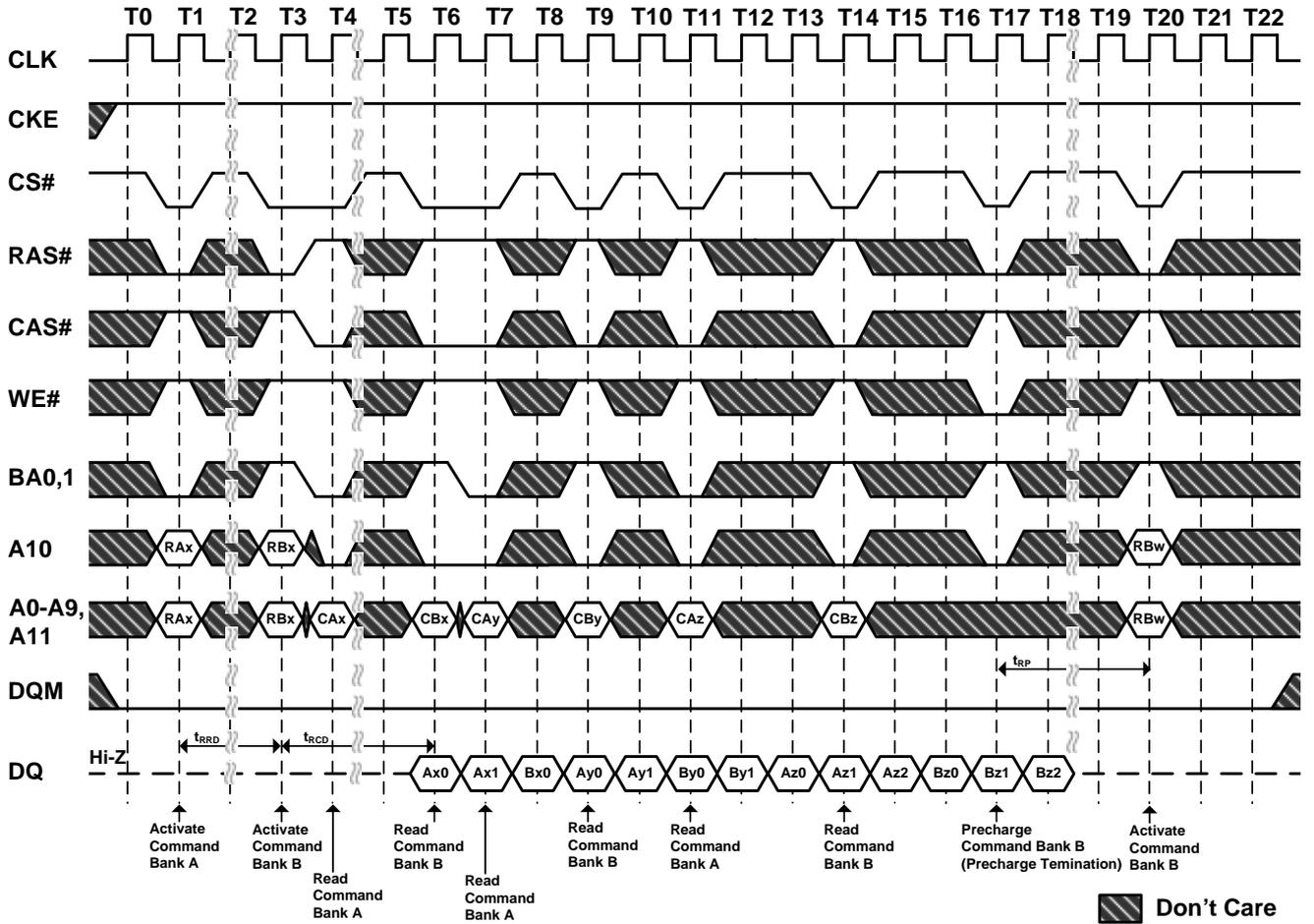
**Figure 42. Precharge Termination of a Burst**
