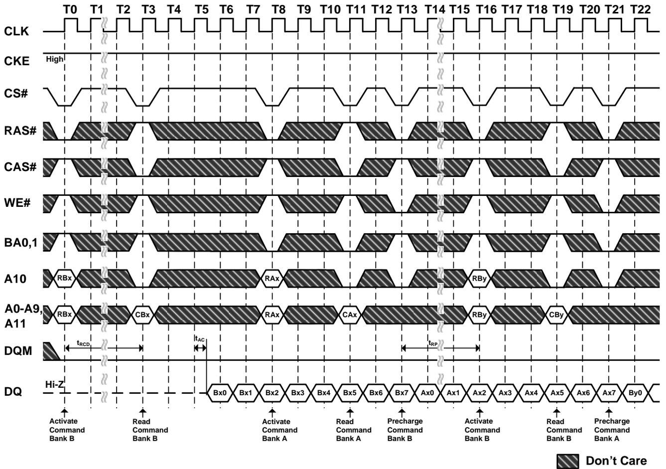
**Figure 30. Random Row Write (Interleaving Banks)**
