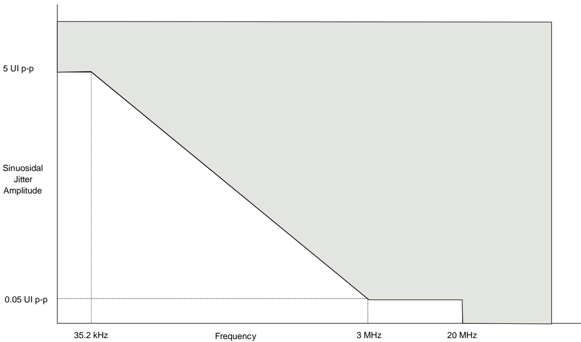
Figure 22: QSGMII single-frequency sinusoidal jitter limits
