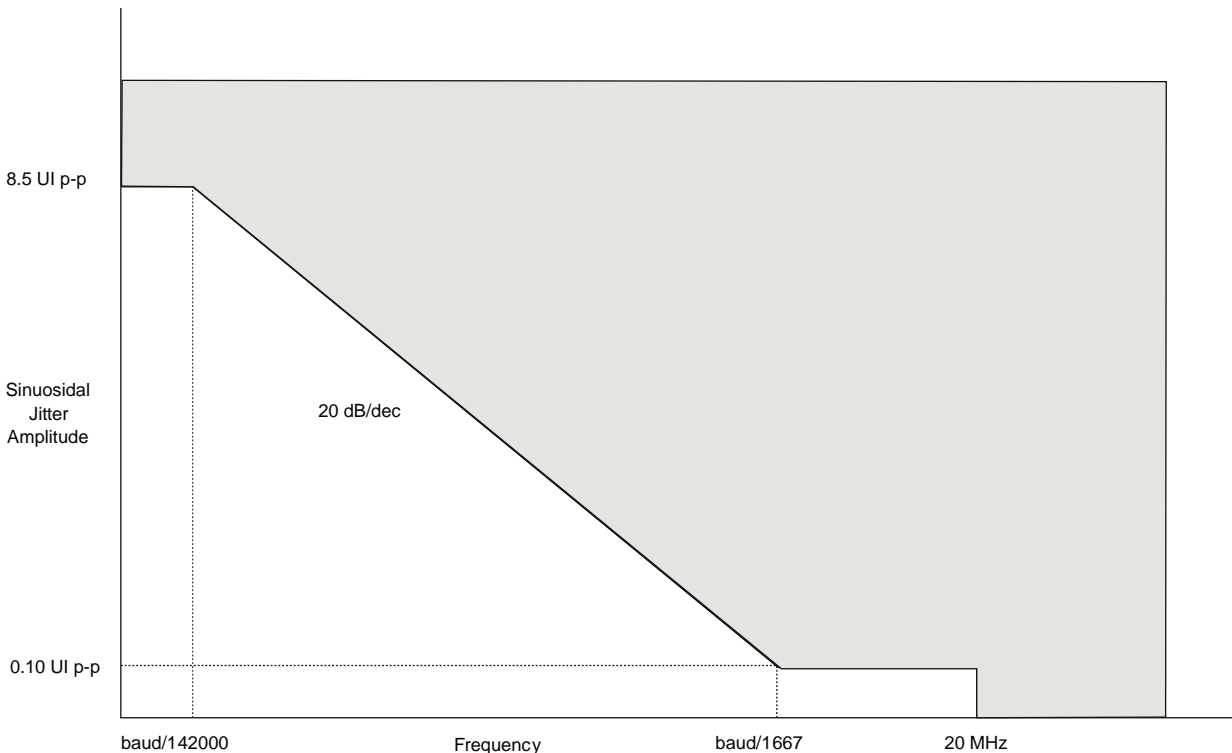
Figure 21: Single-frequency sinusoidal jitter limits
