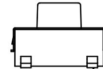
TERMINALS TO BE COLPLANAR WITH IN 0.10mm
