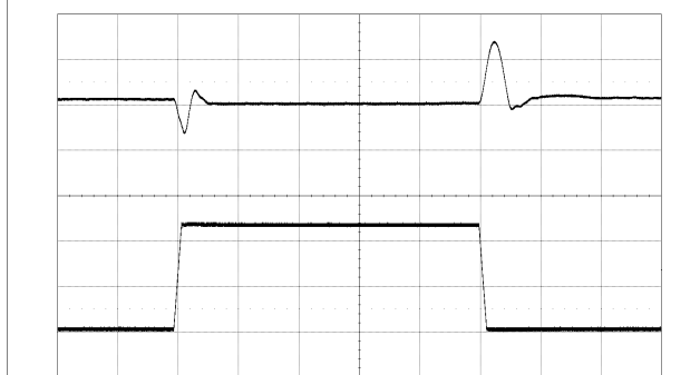
Output voltage response to load current Step-change (12.5-37.5-12.5 A) at: T_{P1} = +25 °C, V_I = 12 V, V_O = 1.0 V di/dt = 2 A/ \mu s, f_{sw} = 320 kHz C_O = 470 \mu F/10 m \Omega
