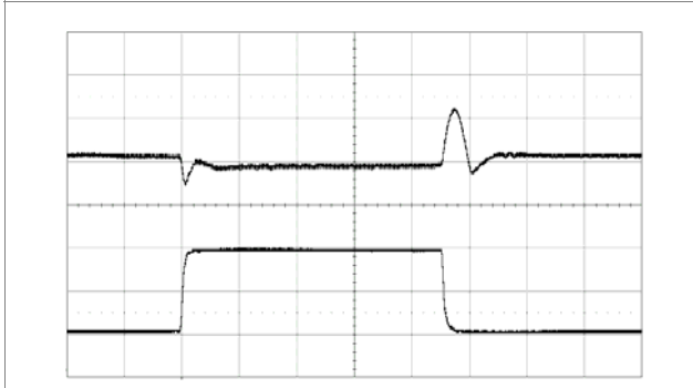
Output Load Transient Response, Default PID/NLR
