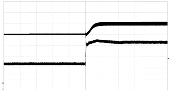
HRR product output at input voltage step 36-75 V, 1 ms/div Bottom trace – input voltage change 36-75 V, 20 V/div Top trace – resulting output voltage change, 1 V/div
