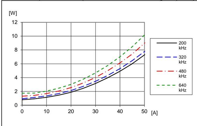
Dissipated power vs. load current and switching frequency at  $T_{P1} = +25\text{ }^{\circ}\text{C}$ ,  $V_I = 12\text{ V}$ ,  $V_O = 1.0\text{ V}$ ,  $C_O = 470\text{ }\mu\text{F}/10\text{ m}\Omega$ . Default configuration except changed frequency
