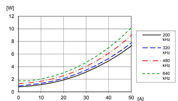
Dissipated power vs. load current and switch frequency at
