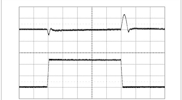
Output voltage response to load Step-change (12.5-37.5-12.5 A) at:
