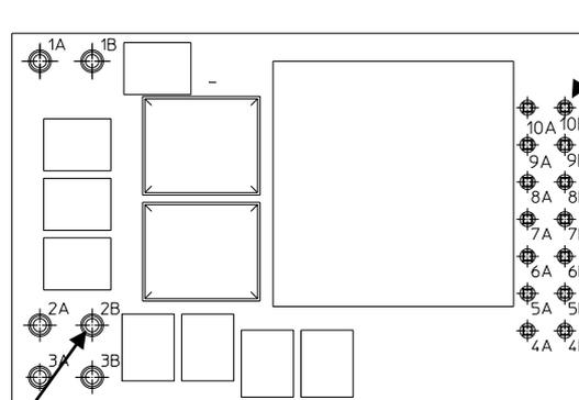
Pin 2B for measurement of minimum Pin (solder joint) temperature  $T_{PIN}$
