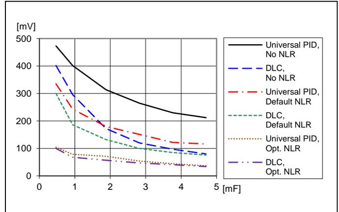
Load transient peak voltage deviation vs. decoupling capacitance. Step (12.5-37.5-12.5 A). Parallel coupling of capacitors with  $470\text{ }\mu\text{F}/10\text{ m}\Omega$ ,  $T_{P1} = +25\text{ }^{\circ}\text{C}$ .  $V_I = 12\text{ V}$ ,  $V_O = 1.0\text{ V}$ ,  $f_{sw} = 320\text{ kHz}$ ,  $di/dt = 2\text{ A}/\mu\text{s}$
