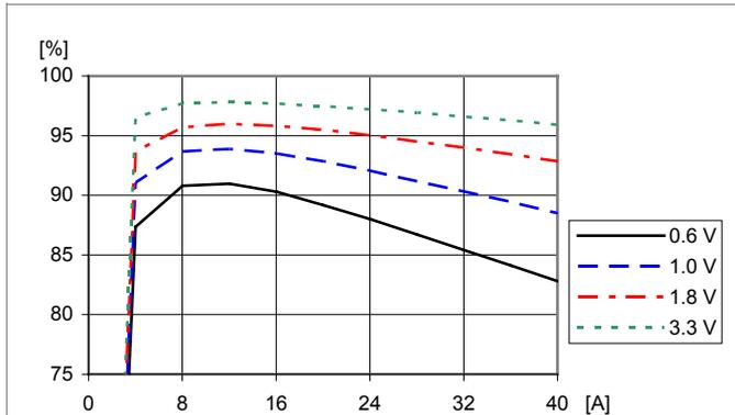
Efficiency vs. load current and output voltage:
