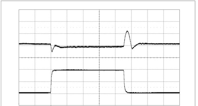
Output voltage response to load current step-change (10-30-10 A) at:
