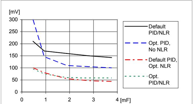
Load transient peak voltage deviation vs. external capacitance.
