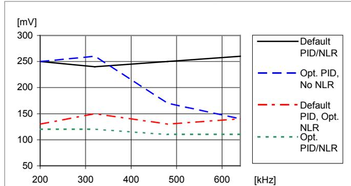
Load transient peak voltage deviation vs. frequency.
