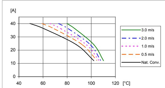
Available load current vs. ambient air temperature and airflow at  $V_O=1.8\text{ V}$ ,  $V_I=12\text{ V}$ . See Thermal Consideration section.
