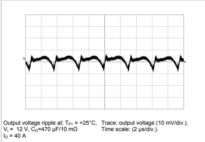
**Output Ripple & Noise,  $V_O=3.3\text{ V}$**
