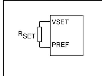
Using an external Pin-strap resistor,  $R_{SET}$ , the output voltage can be set in the range 0.6 V to 3.3 V at 28 different levels shown in the table below. The resistor should be applied between the VSET pin and the PREFERRED pin.
