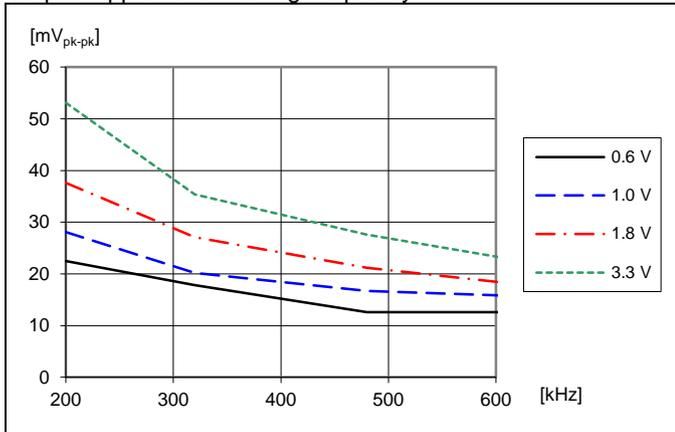
Output voltage ripple  $V_{pk-pk}$  at:  $T_{P1} = +25\text{ }^{\circ}\text{C}$ ,  $V_I = 12\text{ V}$ ,  $C_O = 470\text{ }\mu\text{F}/10\text{ m}\Omega$ ,  $I_O = 50\text{ A}$  resistive load. Default configuration except changed frequency.
