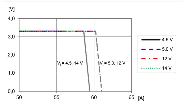
Output voltage vs. load current at  $T_{P1} = +25 ^\circ C$ ,  $V_O = 3.3 V$ .
