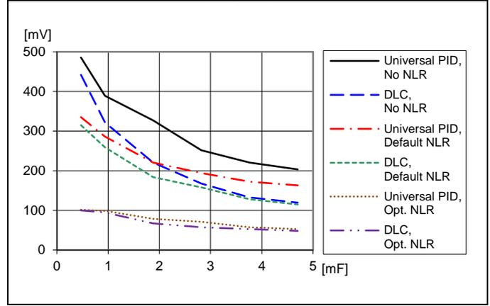
Load transient peak voltage deviation vs. decoupling capacitance. Step (12.5-37.5-12.5 A). Parallel coupling of capacitors with  $470\text{ }\mu\text{F}/10\text{ m}\Omega$ ,  $T_{P1} = +25\text{ }^{\circ}\text{C}$ .  $V_I = 12\text{ V}$ ,  $V_O = 3.3\text{ V}$ ,  $f_{sw} = 320\text{ kHz}$ ,  $di/dt = 2\text{ A}/\mu\text{s}$
