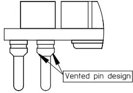
NOTE: Alternative pin option designed for 50A solution with vented pin and Au plating
