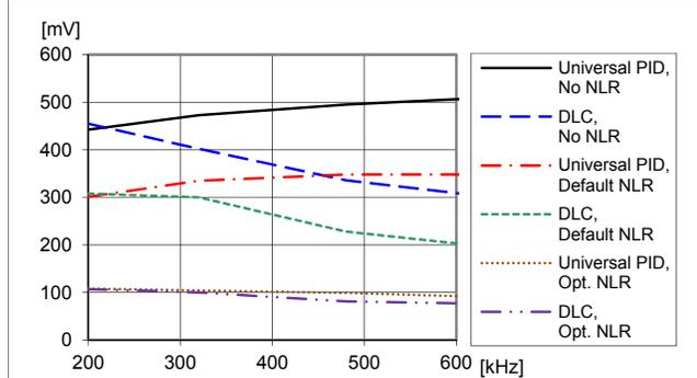
Load transient peak voltage deviation vs. frequency.
