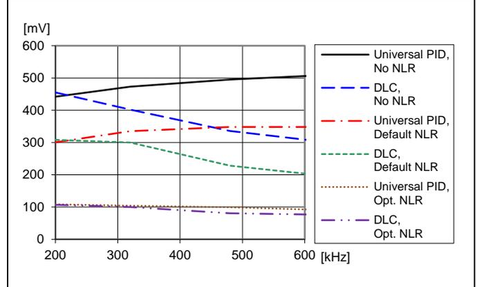
Load transient peak voltage deviation vs. frequency. Step-change (12.5-37.5-12.5 A).  $T_{P1} = +25\text{ }^{\circ}\text{C}$ ,  $V_I = 12\text{ V}$ ,  $V_O = 1.0\text{ V}$ ,  $C_O = 470\text{ }\mu\text{F}/10\text{ m}\Omega$
