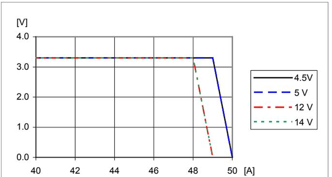
Output voltage vs. load current at  $T_{P1} = +25^\circ\text{C}$ .  $V_O=3.3\text{ V}$ .
