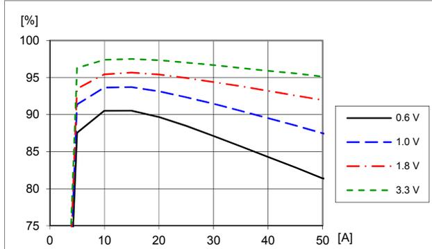
Efficiency vs. load current and output voltage:
