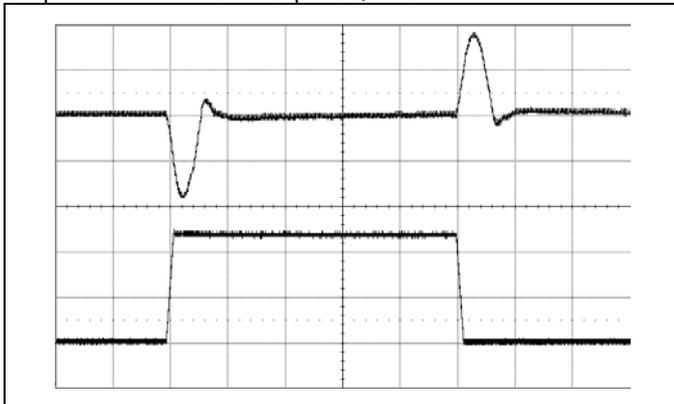
Output voltage response to load current step-change (12.5-37.5-12.5 A) at:
