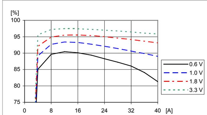
Efficiency vs. load current and output voltage:
