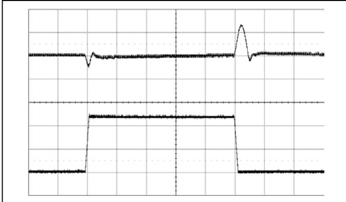
Output voltage response to load current step-change (12.5-37.5-12.5 A) at:
