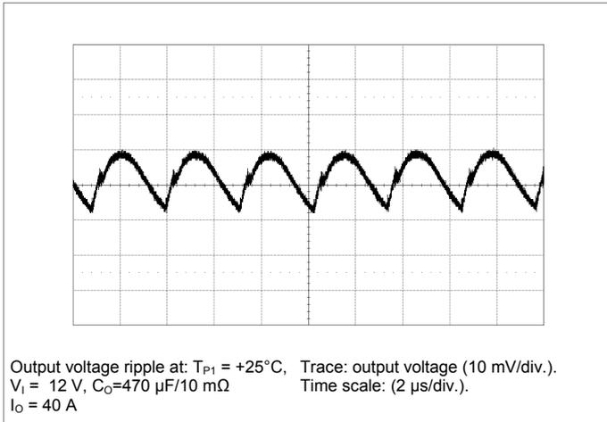
**Output Ripple & Noise,  $V_O=3.3\text{ V}$**
