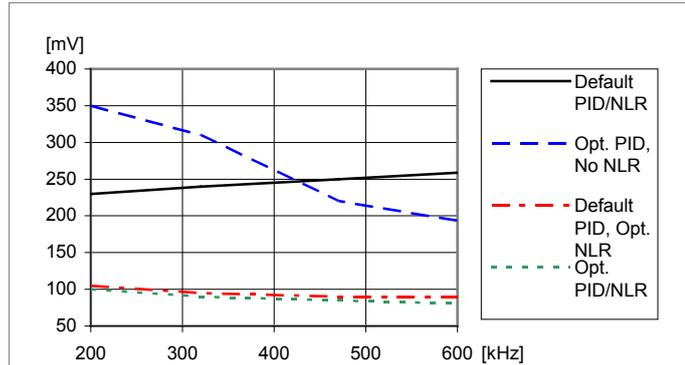
Load transient peak voltage deviation vs. frequency.
