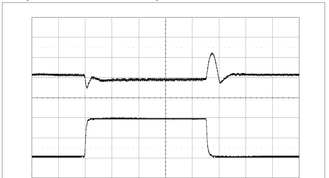
Output voltage response to load current step-change (10-30-10 A) at: T_{P1} = +25^\circ C, V_I = 12 V, V_O = 1.0 V di/dt=2 A/ \mu s, f_{sw}=320 kHz, C_O=470 \mu F/10 m \Omega
