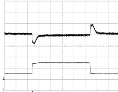
Output voltage response to load current step- change (9.5 – 28.5 – 9.5 A) at: T_{ref} = +25^{\circ}\text{C} , V_I = 53\text{ V} , C_o = 3.8\text{ mF}
