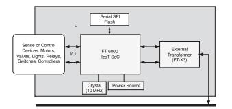
Figure 4: Typical LONWORKS based device
