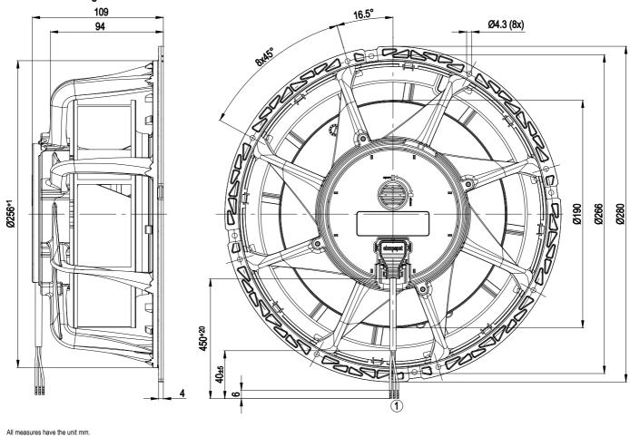
Connection line AWG20, 3x brass lead tips crimped
