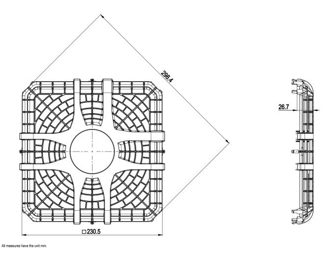
Accessory part: Guard grille 25001-2-2929 intake side, not included in scope of delivery
