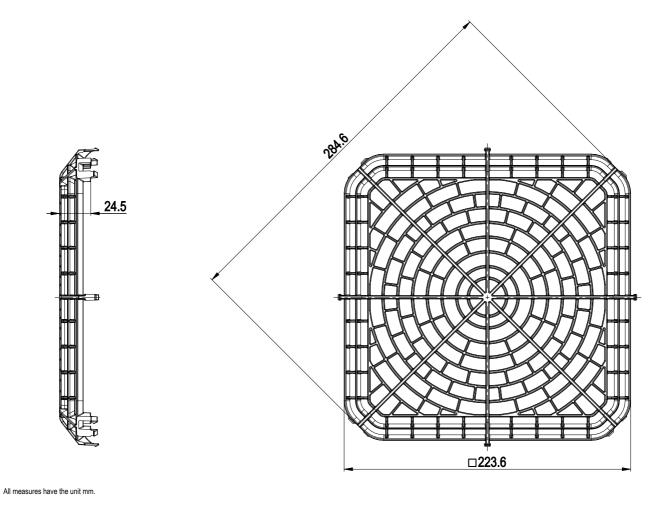
Accessory part: Guard grille 25000-2-2929 outlet side, not included in scope of delivery
