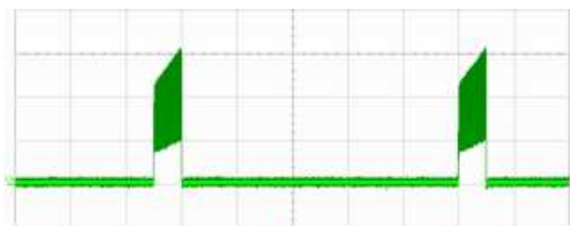
Locked rotor current @ 24 V (I = 0,2A/div ; t = 1s/div)
