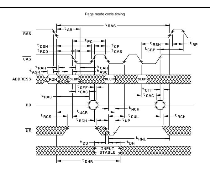
FIGURE 3. <u>Switching waveforms</u> - continued.
