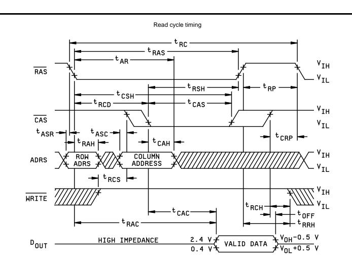
FIGURE 3. Switching waveforms.
