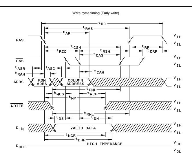
FIGURE 3. Switching waveforms - continued.
