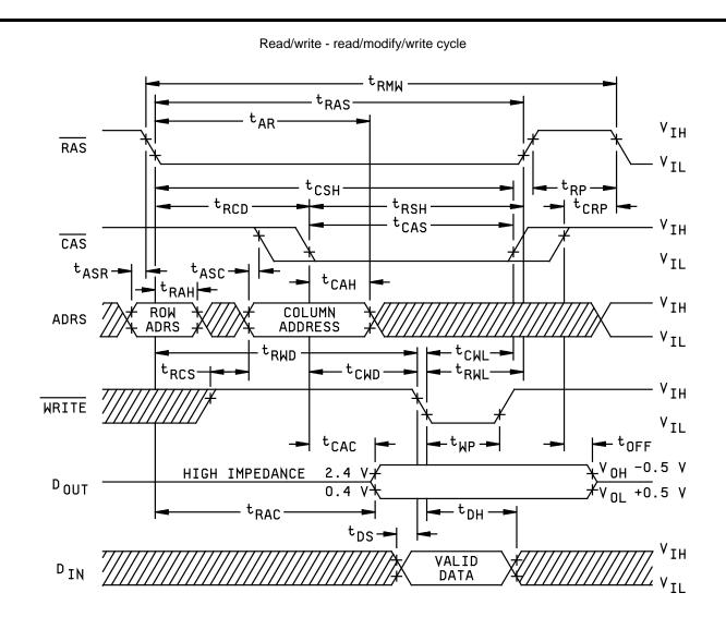
FIGURE 3. Switching waveforms - continued.
