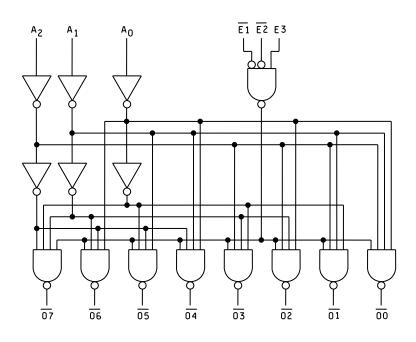
FIGURE 3. Logic diagram.
