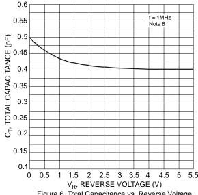
Figure 6 Total Capacitance vs. Reverse Voltage
