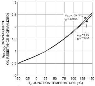
Figure 6 On-Resistance Variation with Temperature
