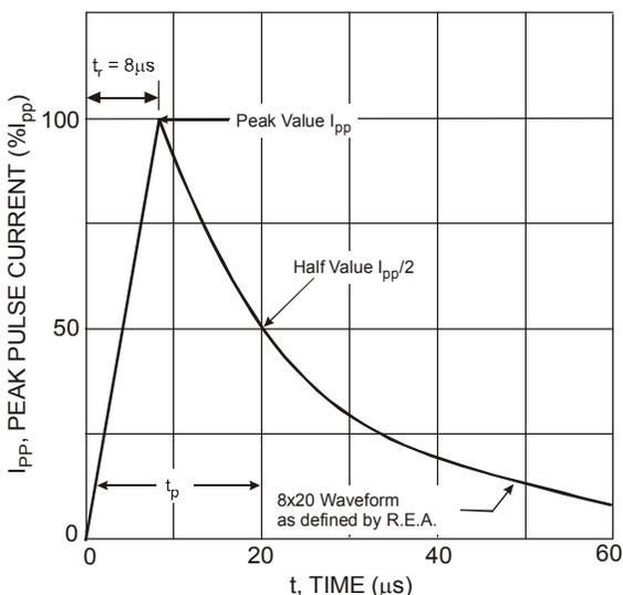
Figure 1 Pulse Waveform
