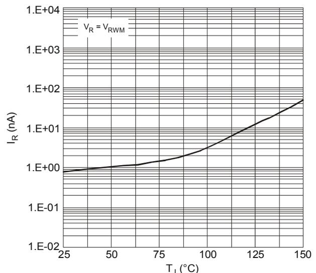
Figure 8 Leakage Current vs. Junction Temperature (typical values)
