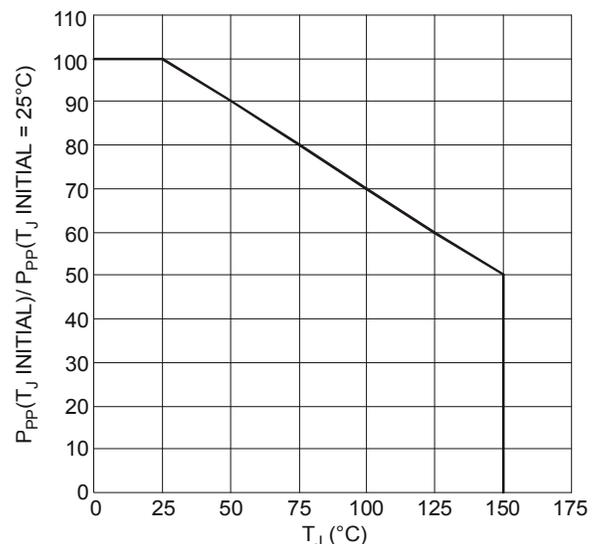
Figure 2 Peak Power Dissipation vs. Initial Junction Temperature
