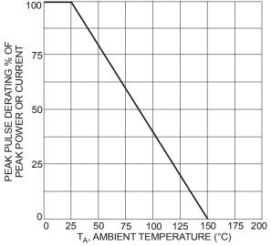
Figure 2 Power Dissipation vs. Ambient Temperature
