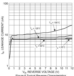
Figure 6 Typical Reverse Characteristics
