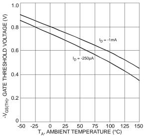
Figure 9 Gate Threshold Variation vs. Ambient Temperature
