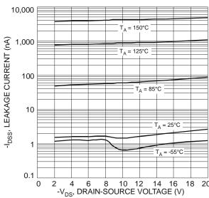
Figure 12 Typical Leakage Current vs. Drain-Source Voltage
