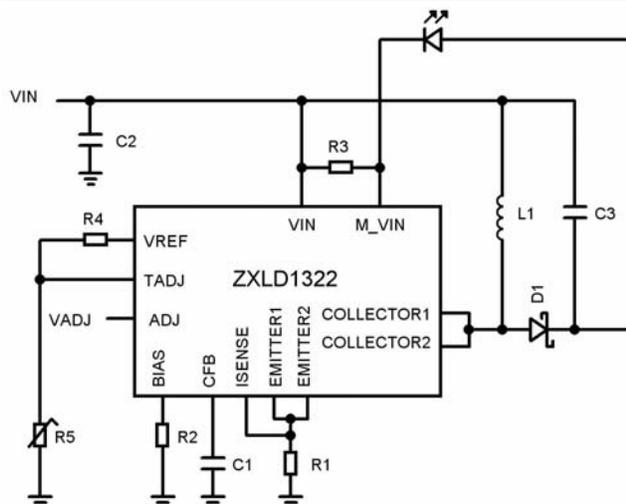
Notes: #. Using standard external components as specified under electrical characteristics. Efficiency is dependent upon external component types and values. Higher efficiency is possible with alternative coils.
