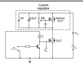
Gate charge test circuit
