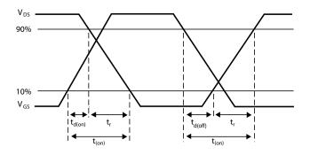
Switching time waveforms
