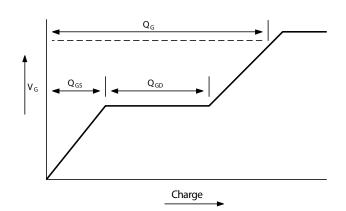
Basic gate charge waveform
