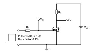
Switching time test circuit
