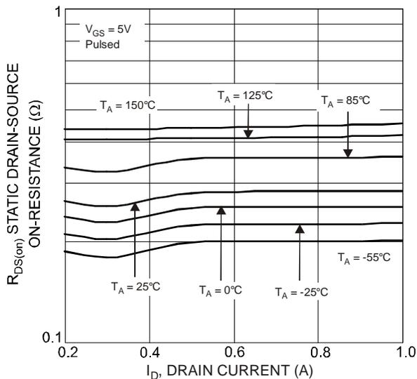
Fig. 5 Static Drain-Source On-Resistance vs. Drain Current
