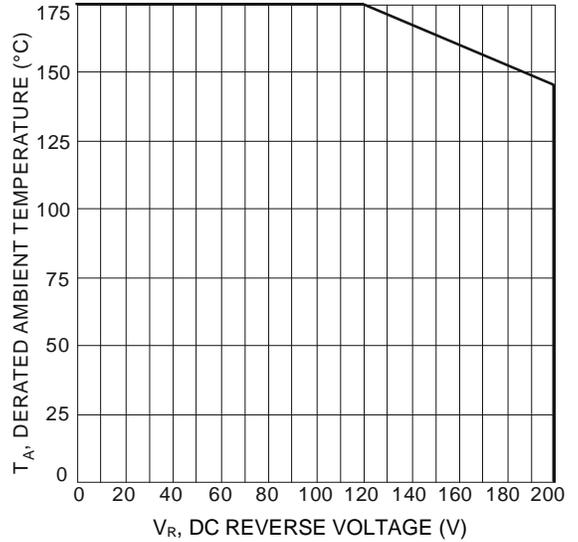
Fig. 8 Operating Temperature Derating
