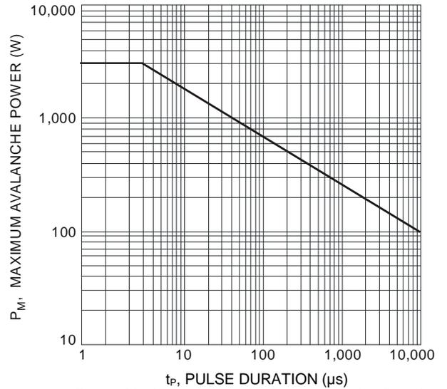
Fig. 10 Maximum Avalanche Power vs. Pulse Duration
