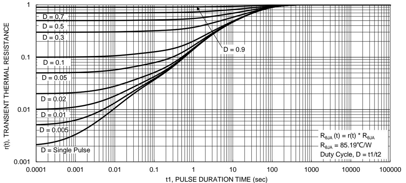
Figure 11. Transient Thermal Resistance
