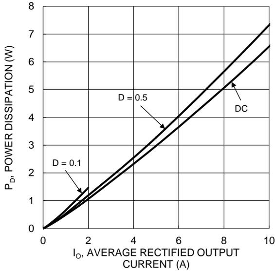
Fig. 3. Forward Power Dissipation  $T_J = 125^\circ\text{C}$
