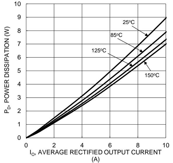
Fig. 4. Forward Power Dissipation  $D = 0.5$
