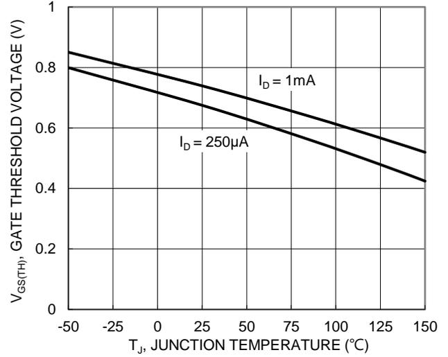
Figure 8. Gate Threshold Voltage vs. Junction Temperature
