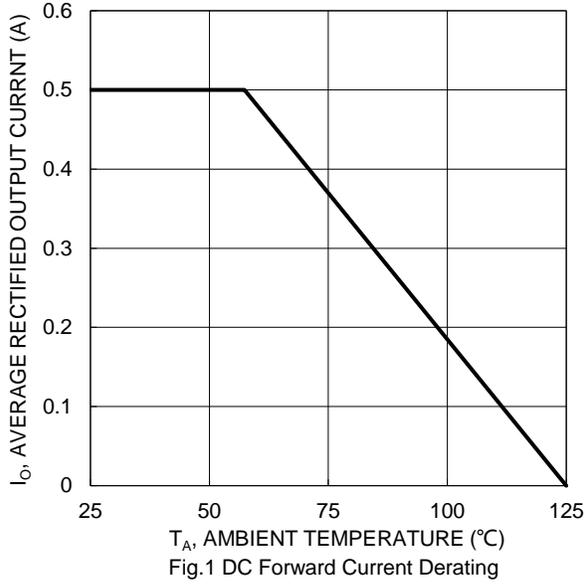
Fig. 1 DC Forward Current Derating
